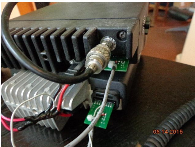
This is the end result, and showing the CDM receiving a signal and making the GM300 re-transmit it.
